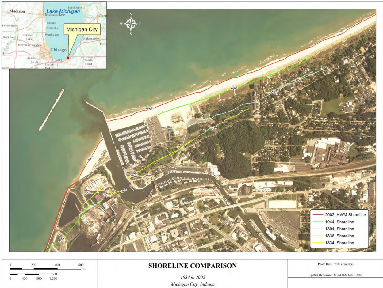
Figure D.3.7-5: History of Fillet Beach Growth at Michigan City, Indiana
