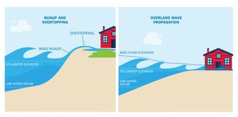
Overtopping is calculated in terms of the amount of water that flows over the barrier crest—the "overtopping rate"
