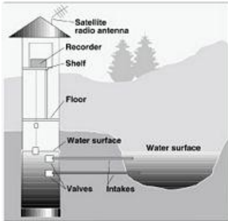
Figure 4: Typical Modern USGS Stream Gage
